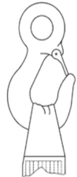
Figure 1: Inadequate accommodation of a webbing eye on a hook of too small radius
